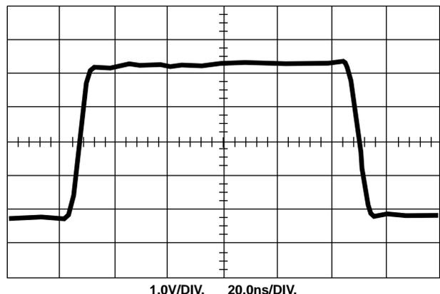
FIGURE 6. OUTPUT WAVEFORM ( $C_L = 18pF$ )
