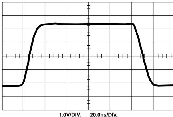
FIGURE 5. OUTPUT WAVEFORM ( $C_L = 40pF$ )
