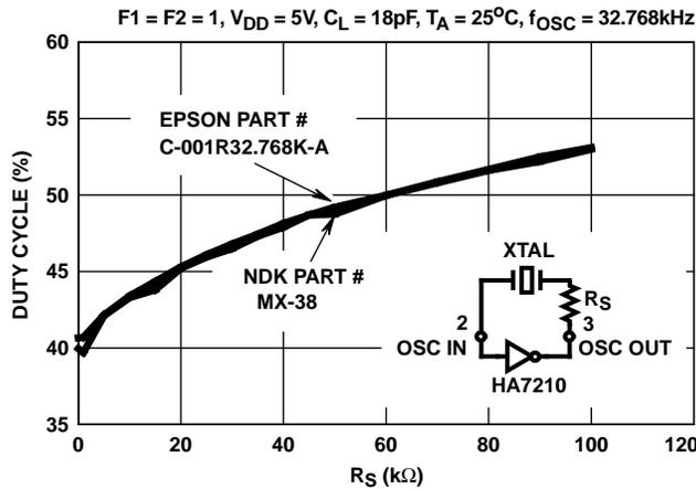
NOTE: Figure 39 (Duty Cycle vs  $R_S$  at 32kHz) should only be used for 32kHz crystals.  $R_S$  may be used at other frequencies to adjust Duty Cycle but experimentation will be required to find an appropriate value. The  $R_S$  value will be proportional to the effective series resistance of the crystal being used.
