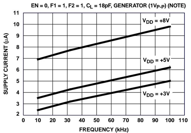
FIGURE 18. DISABLED SUPPLY CURRENT vs FREQUENCY
