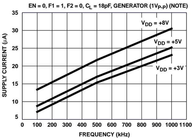
FIGURE 17. DISABLED SUPPLY CURRENT vs FREQUENCY
