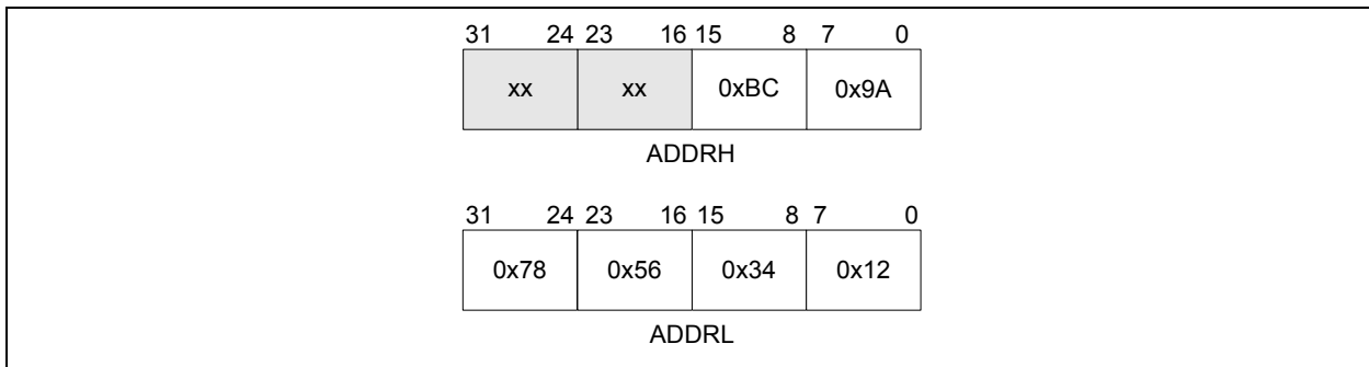
FIGURE 6-1: EXAMPLE ADDRL, ADDRH ADDRESS ORDERING
