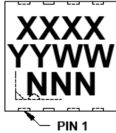
8-Lead DFN (3x3x0.9 mm)
