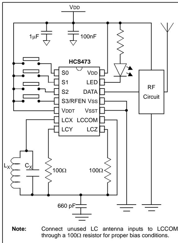
**FIGURE 2-3: S0/S1/S2 PIN DIAGRAM**
