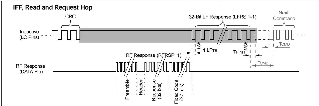
**FIGURE 3-21: LF COMMUNICATION ANALOG DELAYS**
